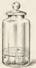
FIG. 46.—Cyanide-jar prepared for use. P , perforated cardboard; C , lumps of cyanide of potash.
